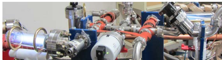
Figure 7. Simultaneous running of two argon plasmas with ring RF electrodes (left) and bar electrodes (back right).
